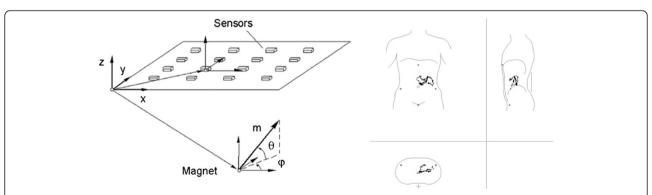
**Figure 1 Magnetic sensor and duodenal arch.** Tracking of the magnetic pill by 16 (4x4) external sensors. The position is defined by coordinates X, Y and Z, and the rotation is defined by the angles  $\varphi$  and  $\theta$  (left). 3D representation pyloric and duodenal passage (right). The sequence displayed is 10 seconds long.
